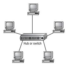
As a general rule, switches are superior to hubs. Hubs mirror all traffic to all computers, whereas switches are smart enough to send packets only to the intended destination. The result is that switches let two pairs of computers
