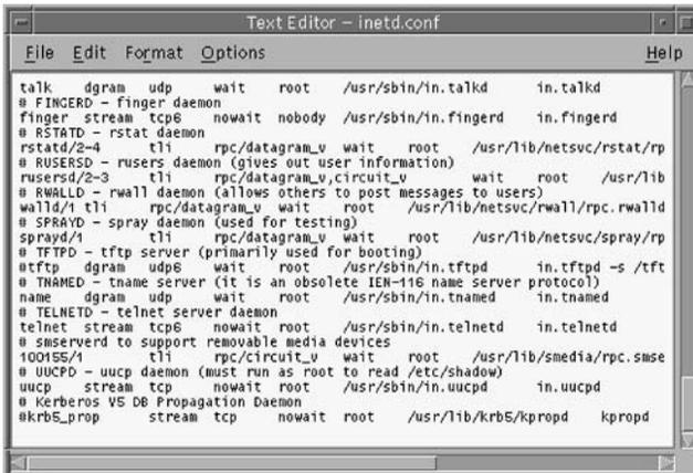
FIGURE 4-1 Entry for tftpd in the inetd.conf file
